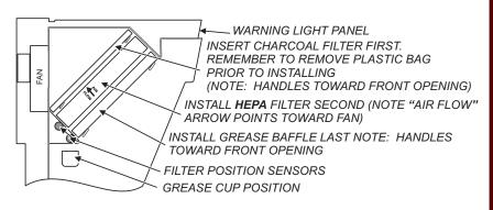
Remove the protective plastic bag from charcoal filter before installing.
